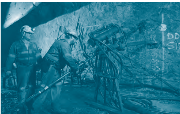
Underground Diamond Drilling
